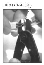
Unplug the wire connection between the two blades (inside silicone tube).
